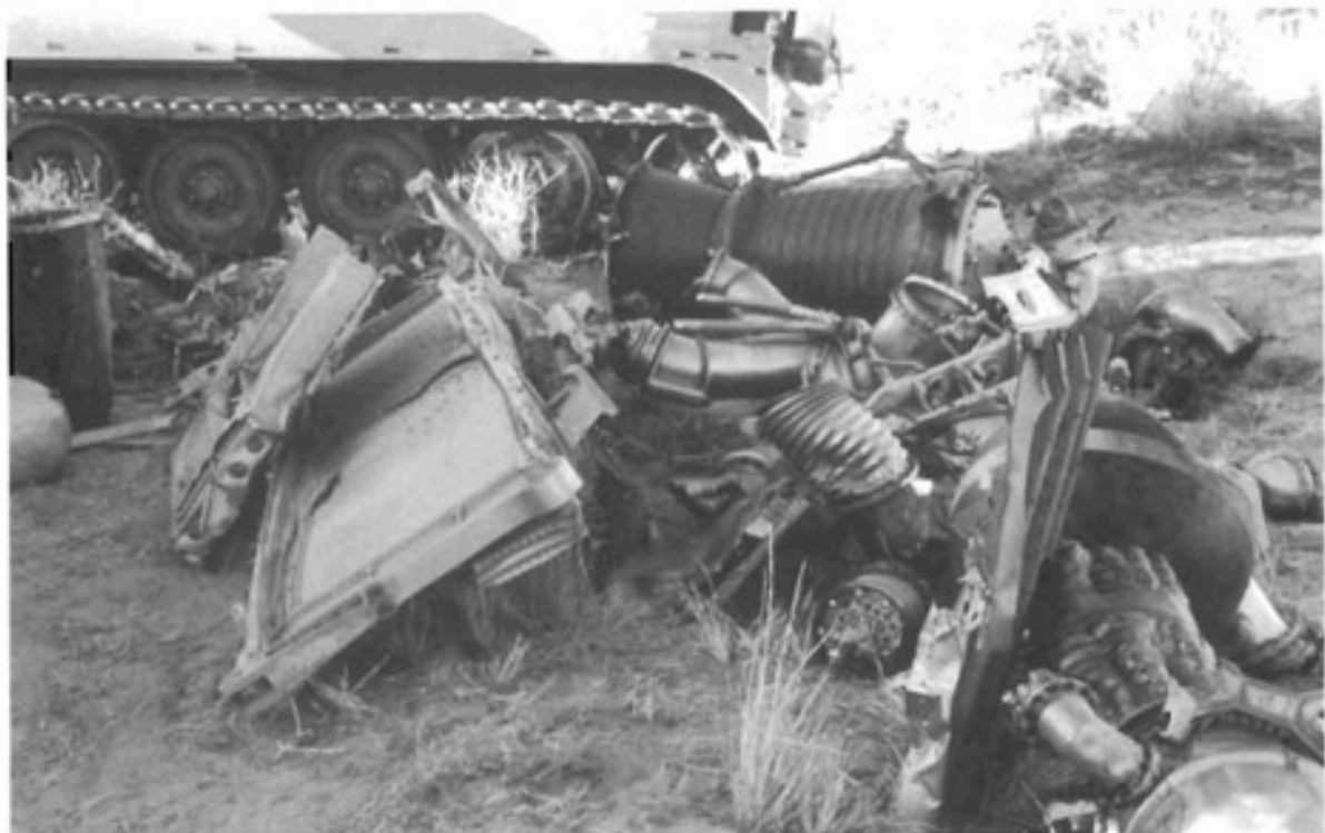
Figure 7 Recovered debris from the Europa F-4 vehicle, indicating the level of damage resulting from the activation of the abort system. Unlike the Wresat Redstone, the F-4 remains were in a highly fragmented state. (Roger Hentwood)
