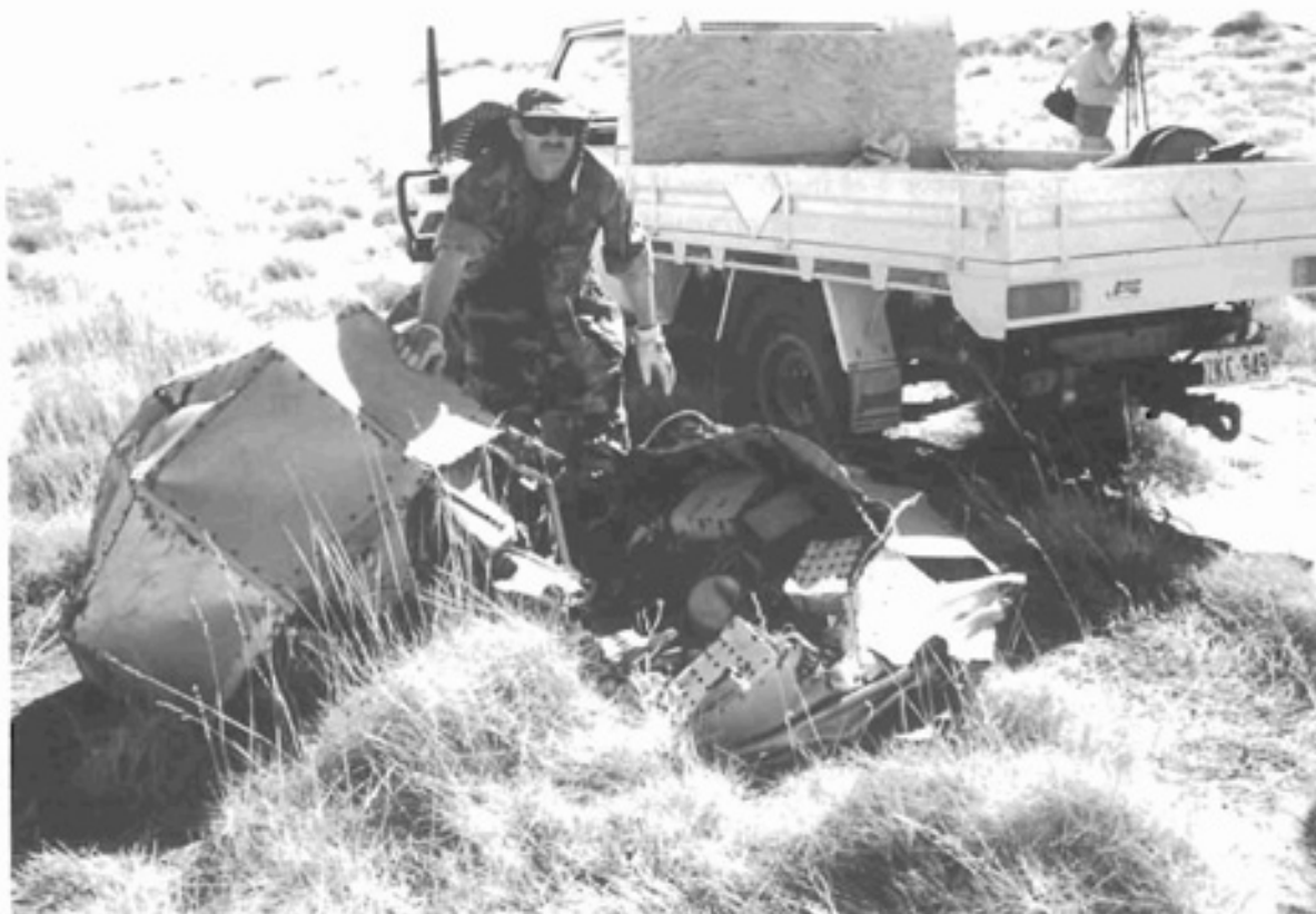
Figure 8 The Europa F-5 dummy satellite, as found. Although the casing had split open on impact, the contents were intact and in good condition. (Roger Hentwood)
