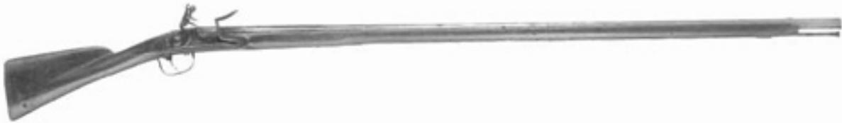
*Figure 1 American-made composite musket from the Revolutionary War, assembled with a barrel bearing London proofmarks, a lock bearing French marks and the trigger and stock of an American manufacturer. (National Museum of American History)*
